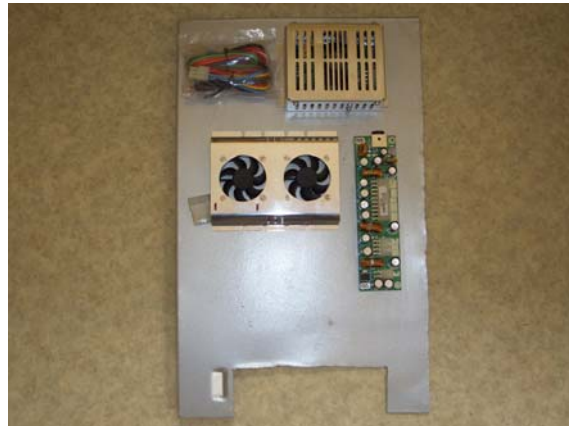
Before Cutting Any Holes Check Where Components Can Go
