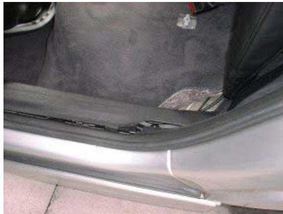
Look For Existing Cable Runs
