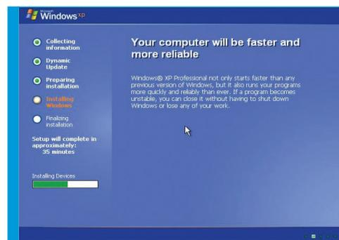
**3** This is the easy part of the installation. Much of the install is the same as building a new PC. It's worth running ScanDisk and Disk Defragmenter a few times once your Windows installation has been completed, to ensure the disk is optimised for smooth performance.
