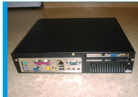
**6** With the system setup complete, copy your media files to your system. If you want to connect your CarPC to your home PC using a direct Ethernet cable connection and without using a network hub in between them, you'll need a crossover cable.
