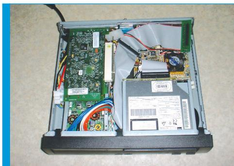
**2** You don't have to think small, as all installations are different, but it helps. We're using a Cubid 2688R case with a VIA mini-ITX board. This case doesn't leave much room inside, but by using smaller components, such as a laptop hard drive, you can pack quite a bit more in.
