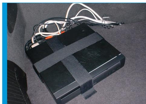
**9** You don't want your equipment to move around while you're driving. The easiest way to prevent this is to use Velcro, which sticks to the carpet or another strip of Velcro. The cables are then tied and secured underneath the carpet for neatness.
