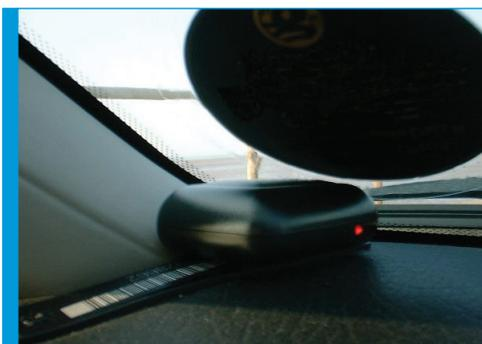
**11** Ensure your GPS receiver is compatible with your intended application. eBay is a good source of USB GPS units, which, when used with a USB hub in the dash, make things easier in terms of cabling. If your car has heat-reflective film in the windows, this can affect the quality of the signal.
