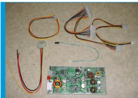
**14** There are several options for powering your system, but it's widely recognised that the power supply from Opus Solutions is among the best. It controls the startup and shutdown of the system, as well as maintaining a stable voltage.
