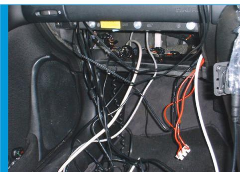
**7** Now to install the system in the car. You'll doubtless have excess cables to stow, along with items such as USB hubs. Space behind the dashboard can be useful here, but be aware of heating or AC elements and don't put anything in there that may be a potential fire risk.
