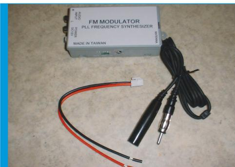
**13** If you have a high-specification car radio, it might have an auxiliary port (possibly left and right phono plug leads), which is the best way to get sound in to your system. Failing this, buy an FM Modulator from eBay for £25-35 – it's easy to connect and all you need to do is tune in your radio.
