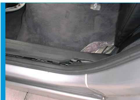
**8** If you put your machine in the boot, you'll need to supply power, audio, video and USB feeds to the rear of the car. Ensure you separate the power cables from the audio feeds to prevent interference. You may want to use a mains three-pin socket and plugs so the system can be quickly removed.
